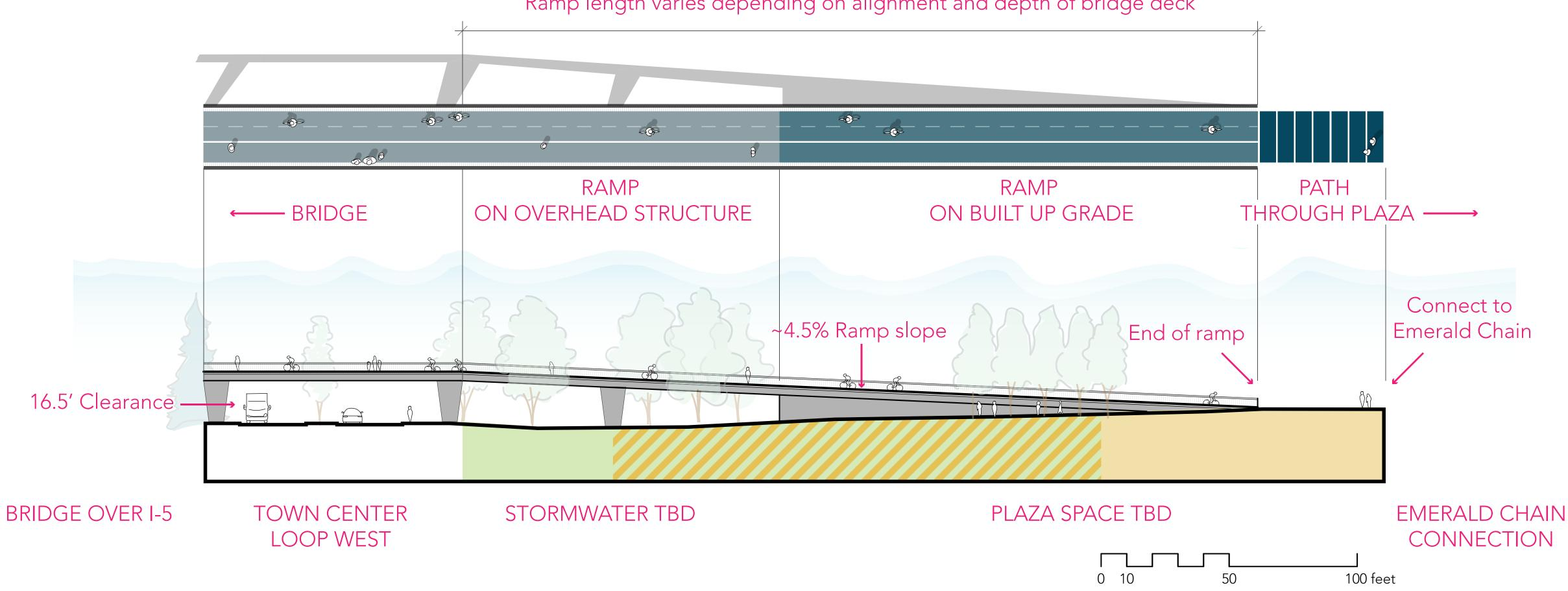
Ramp length varies depending on alignment and depth of bridge deck
