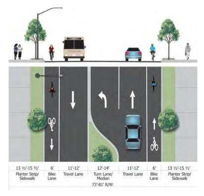
Figure 7: Minor Arterial Cross-Section (Wilsonville TSP)
