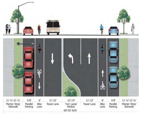
Figure 8: Collector Cross-Section (Wilsonville TSP)
