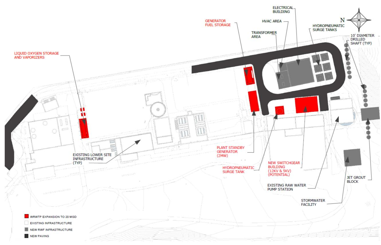
Figure 6.1 WRWTP Site Layout – 20 mgd Capacity
