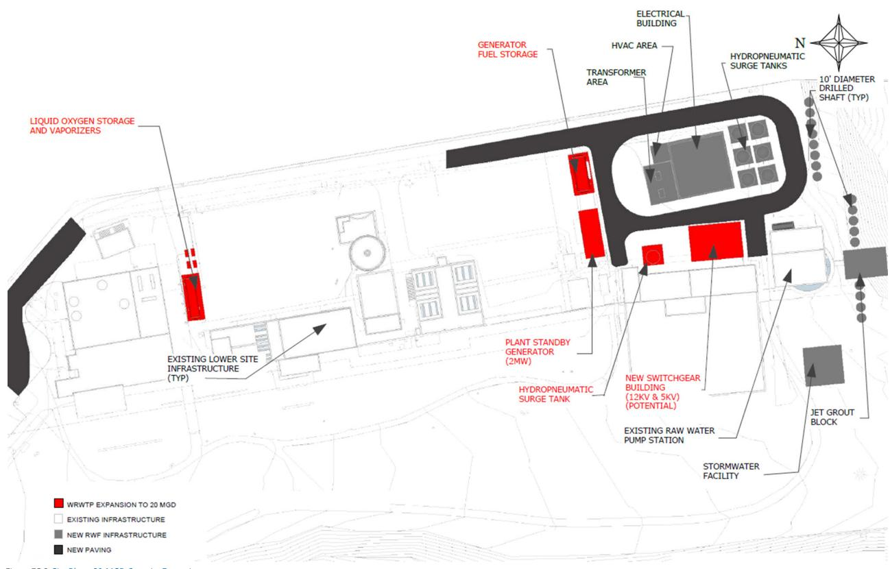
Figure ES.2 Site Plan – 20-MGD Capacity Expansion
