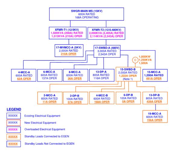
Figure 5.2 Current Electrical Load Diagram
