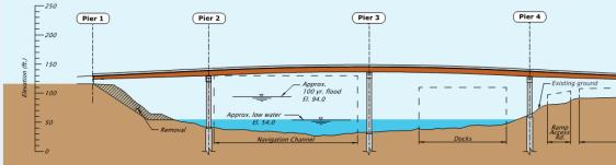
Profile line drawing of Steel Girder bridge
