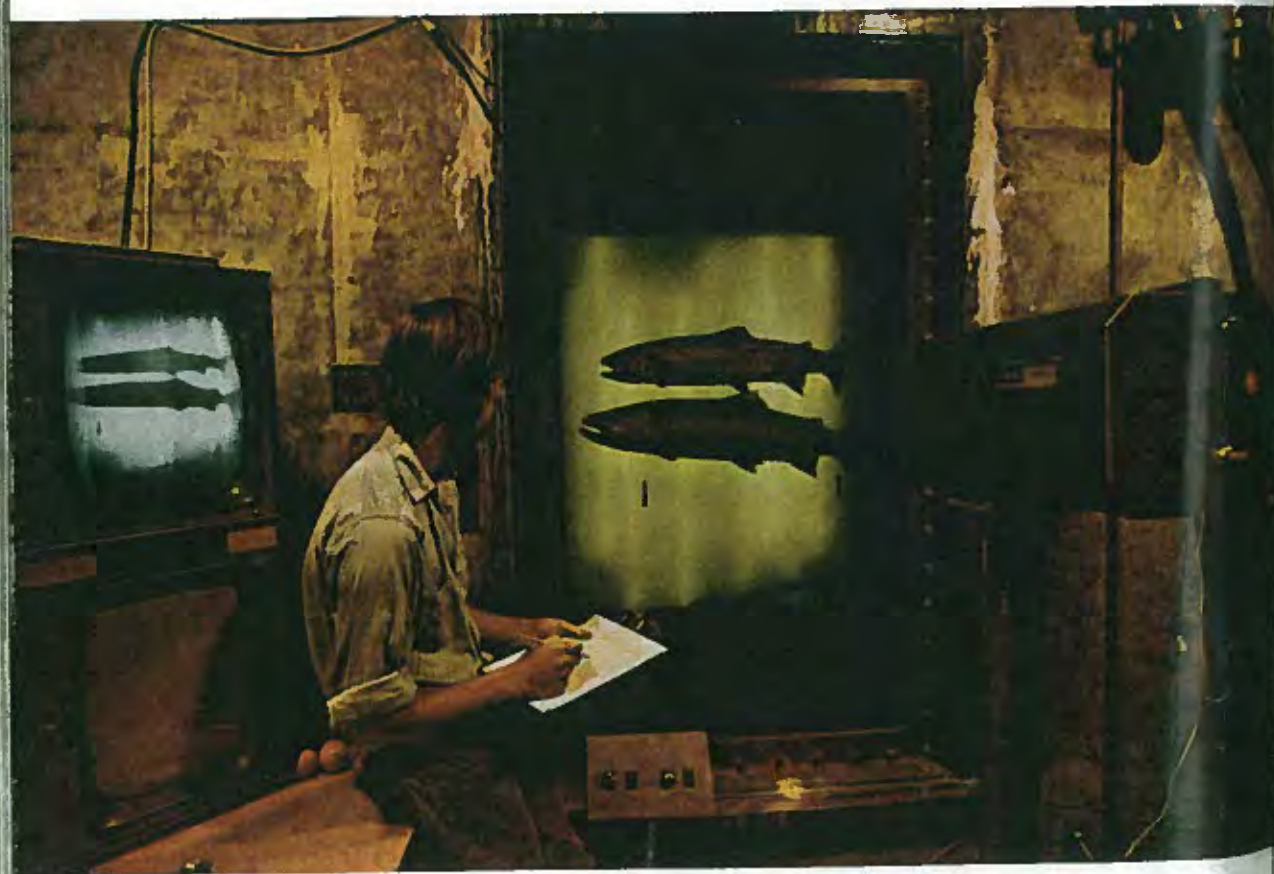
Census of home-bound fish counts swimmers making their way up a new fish ladder at Willamette Falls. Television camera aimed at the underwater window videotapes passersby—here two steelhead trout.
