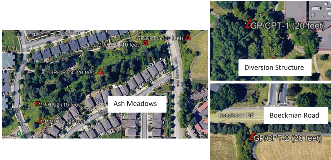
Figure 3. Geotechnical field exploration locations
