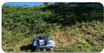
With a remote slope mower, City Road Maintenance crews can safely mow blackberry on dangerous inclines or other hard-to-reach places.
