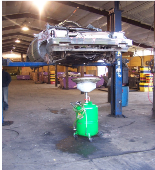
Fluid Gravity Drain System
