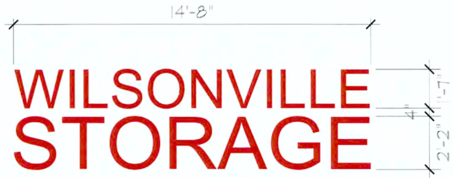
3 SIGNAGE DETAIL - SOUTH ELEVATION SCALE 1/4" = 1'-0"
