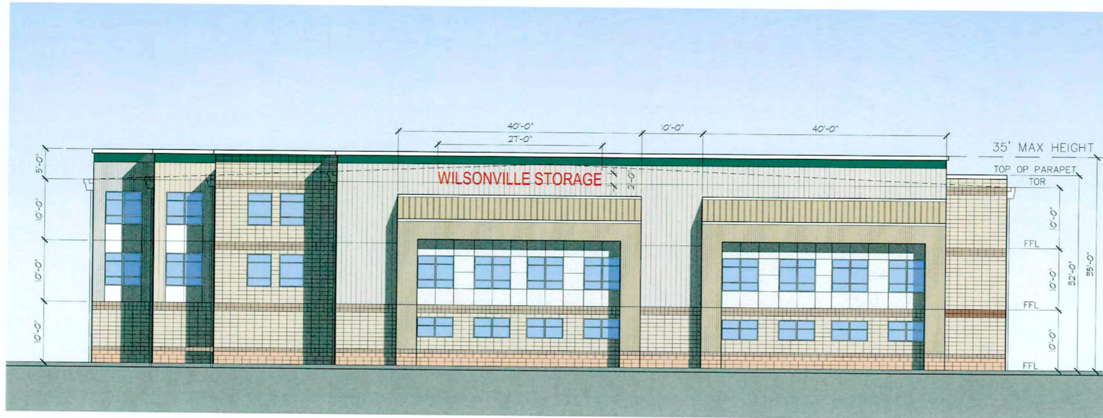
1 SOUTH ELEVATION SCALE 1/8" = 1'-0"
