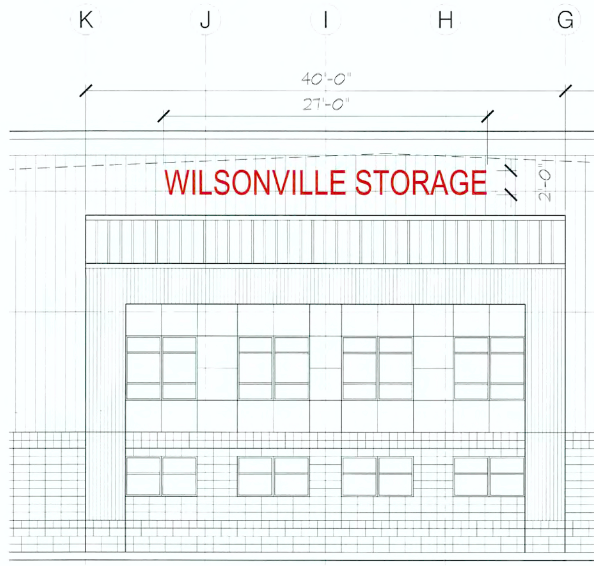
1 SIGNAGE - SOUTH ELEVATION SCALE 1/4" = 1'-0"
