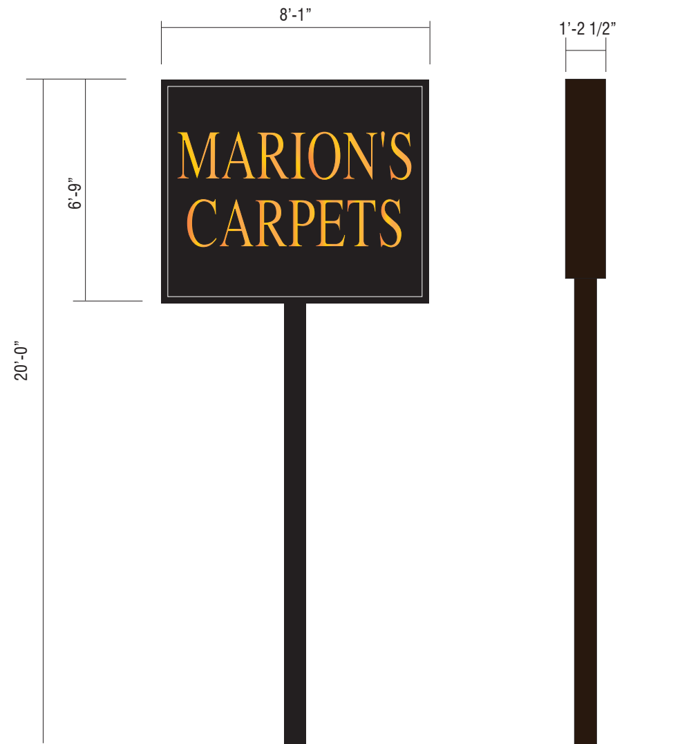
1 Sign #5 - Illuminated Pylon Sign Scale: 1/4" = 1'-0"
