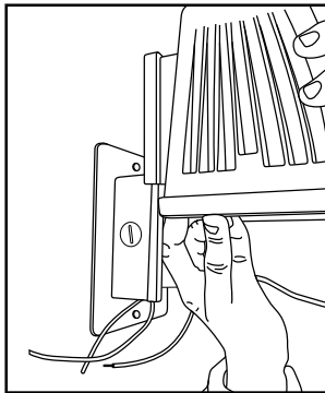
Slide fixture housing onto mounting box
