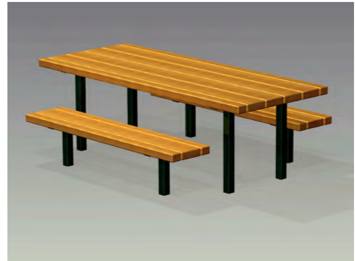
PICNIC TABLE Picnic Table and Seats shall be TimberForm® Parkway series model No. 2062, 7'-10" long and 5'-8" wide. Metal posts and frame to be powdercoat - black. Seat and tabletop shall be kiln dried douglas fir wood. Quantities shown on the project drawings. Manufacturer: Columbia Cascade Company, 1300 SW Sixth Avenue, Suite 310, Portland, OR 97201-3464 U.S.A.
