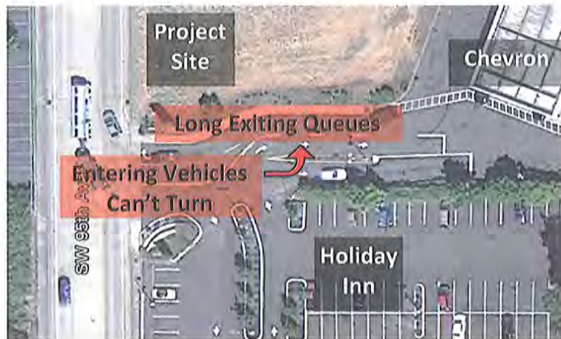
Figure 7: Internal Project Access Concern
