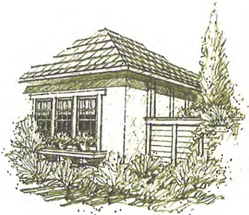
Example of transition from stucco on public street or open space elevation to lap siding stucco board at non-public street or open space elevation
