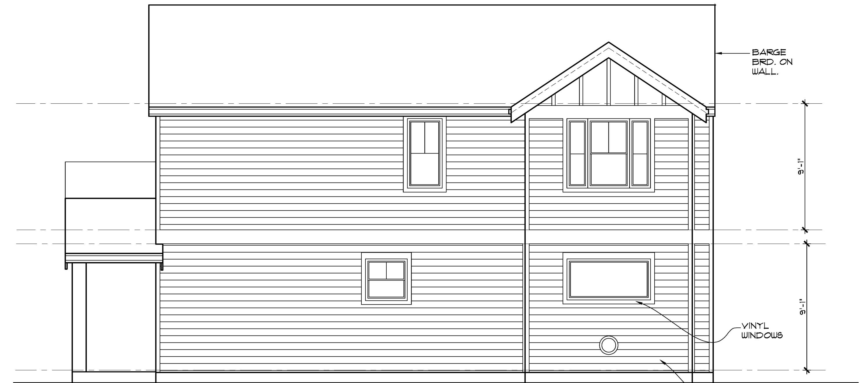
EAST ELEVATION ELEVATION "B"
