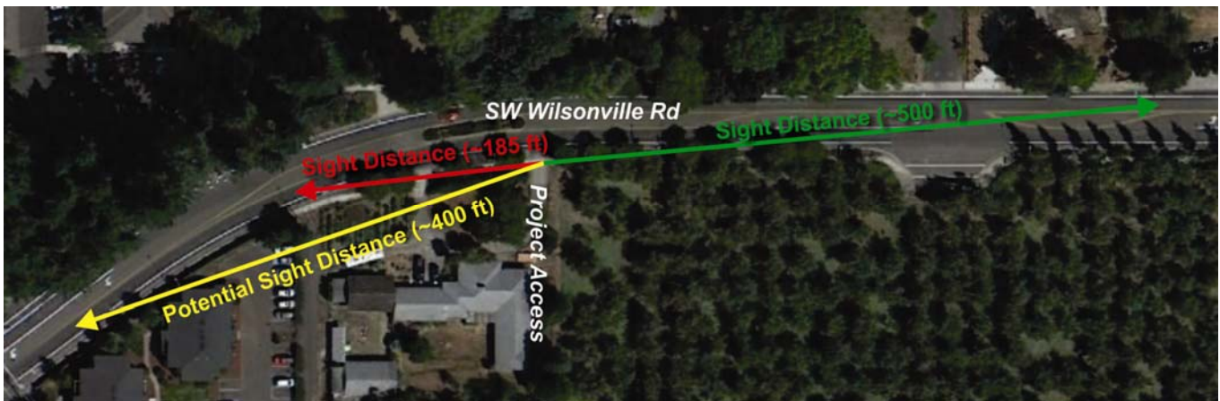
Figure 1: SW Wilsonville Road Sight Distance Analysis Findings
