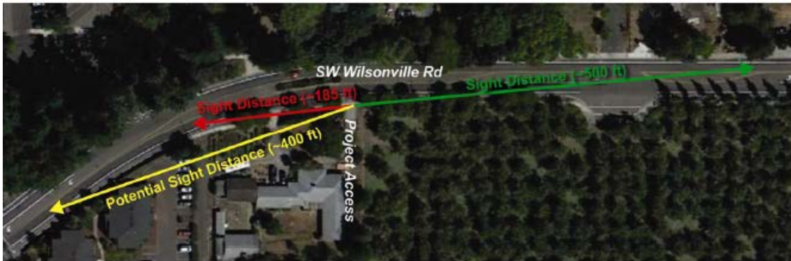
Figure 1: SW Wilsonville Road Sight Distance Analysis Findings
