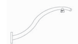
MANUFACTURER: PHILIPS HADCO URBAN LUMINAIRE: WESTBROOK CXF14 POLE: 13' DECORATIVE CAST ALUMINUM ARM: SINGLE (HFP710) FOOTING: AB CHANCE - C11242NG4TK W/ROUND MOUNTING PLATE FINISH: BLACK DARK SKY FRIENDLY HPS PROVIDE AUTO PROFILE DIMMING - COORDINATE PROFILE WITH CITY OF WILSONVILLE AND MANUFACTURE
