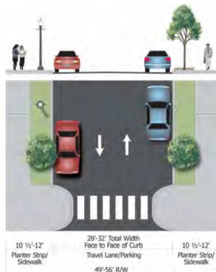
FIGURE 3-9. LOCAL STREET CROSS-SECTION
