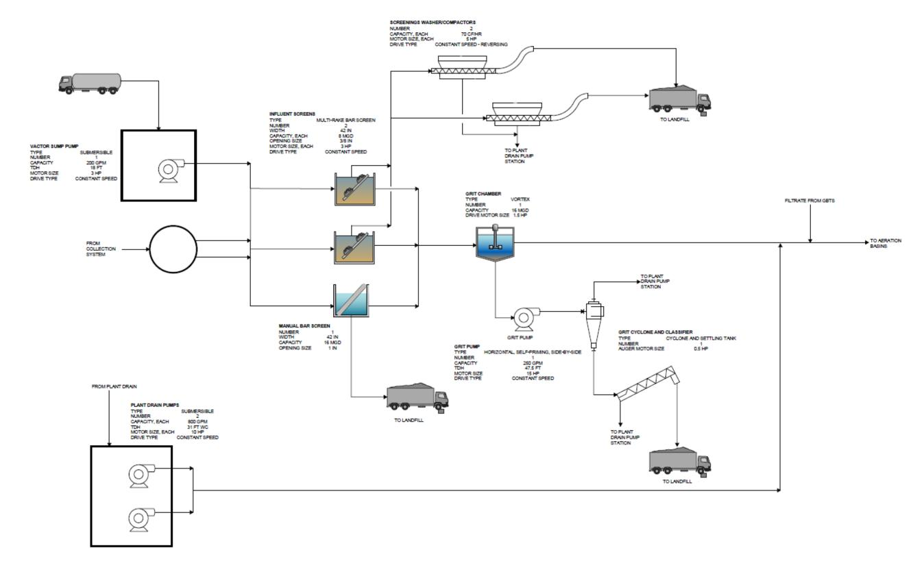
Figure G.1 Preliminary Treatment Schematic
