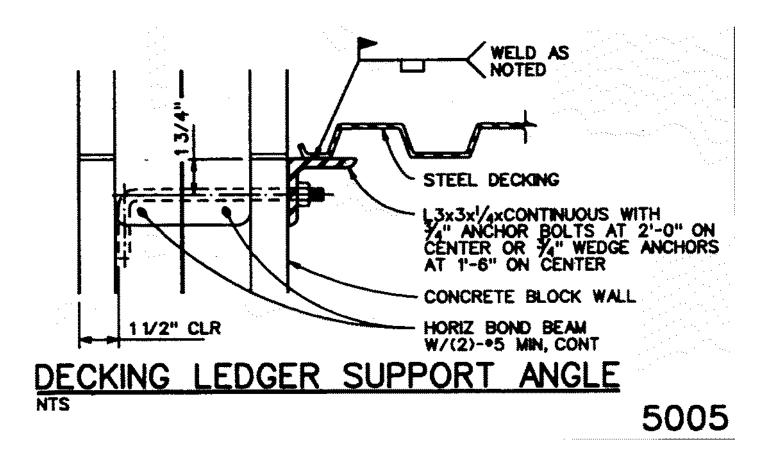
WALL ANCHORAGE CONNECTION DETAIL ALONG NORTH AND SOUTH WALL ELEVATIONS
