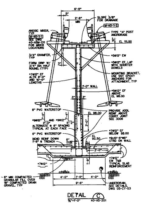
**Dividing Wall Section Reinforcing**
