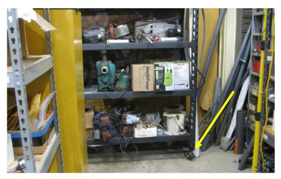
Figure 22 Workshop - Storage Shelving Lacks Restraint to Structure
