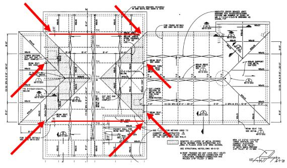
Figure 1.2 Operations Building - Collector Beam Locations and Anchorage Deficiencies
