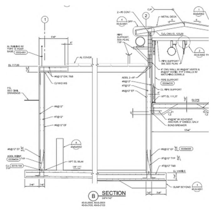
Stabilization Basin Perimeter Wall Section Reinforcing
