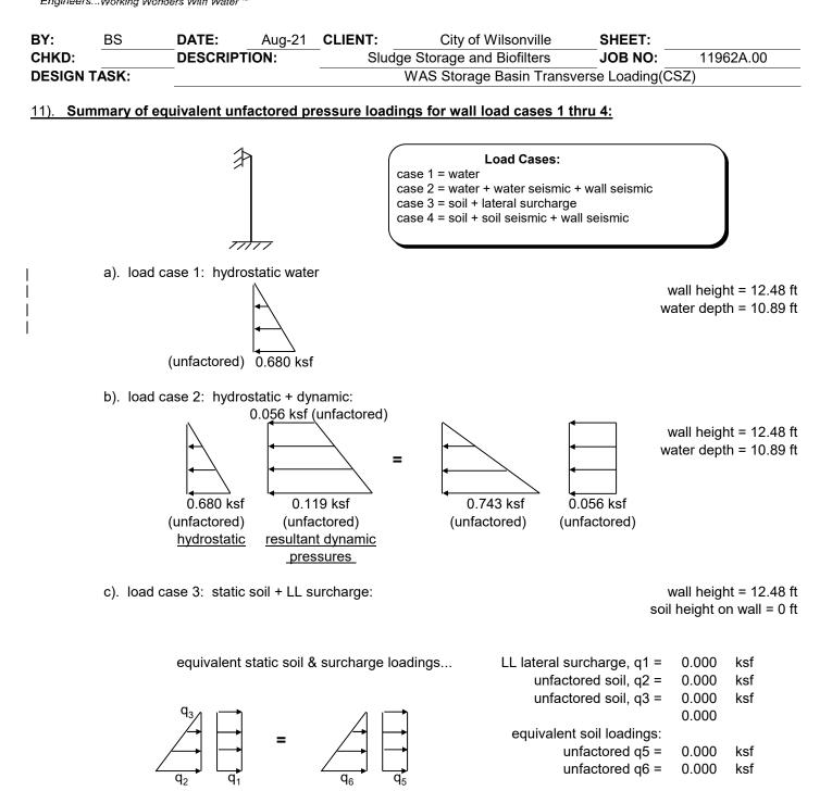
d). load case 4: soil seismic: (\*note: add static soil pressure q6 & q7 to the seismic soil shown below) equivalent seismic soil pressure loading & seismic wall loadings...
