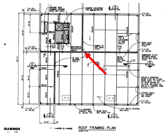
Figure 1.3 Process Gallery - Collector Beam Location and Anchorage Deficiency
