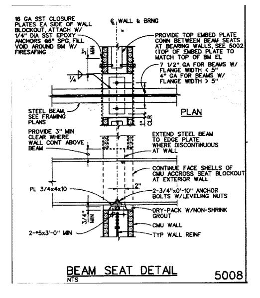
BEAM ANCHORAGE CONNECTION DETAIL ALONG EAST AND WEST WALL ELEVATIONS
