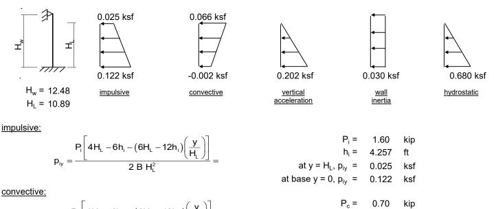
$p_{cy} = \frac{P_{c} \left[ \frac{4H_{L} - 6h_{c} - (6H_{L} - 12h_{c})\left(\frac{y}{H_{L}}\right) \right]}{2 B H_{l}^{2}} =$
