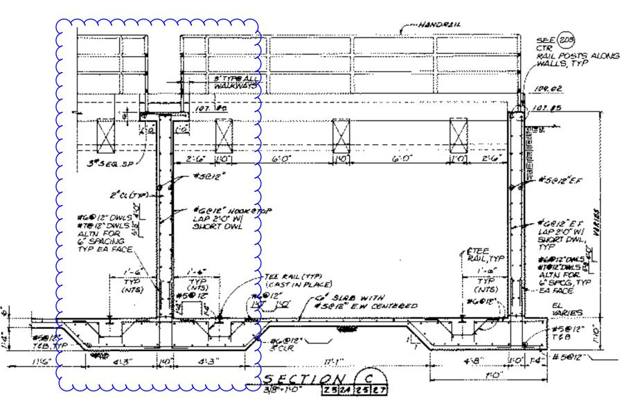
**Dividing Wall Section Reinforcing**
