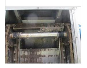
Bar screen rake had several teeth in the rake assembly bent. Would not allow rake to mesh with bar screen.
