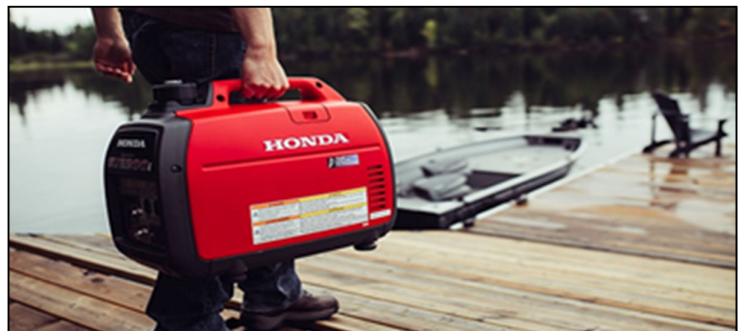
Portable generators like the two shown above must operate outdoors to prevent the dangerous build-up of carbon monoxide gas. They run on unleaded gasoline and require the use of extension cords to get electricity where you need it.
