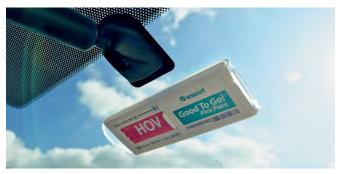
**Image:** Example of a transponder that drivers use in Washington state's modern tolling system.
