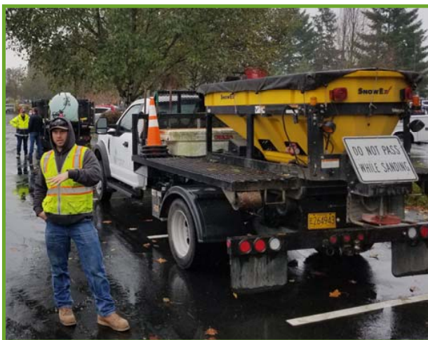
Manny Ghiseline, Roads Maintenance Specialist describing operation of the sanding equipment
