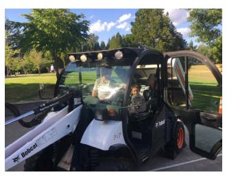
An unusual piece of equipment at the party was the tool cat. This is a multi-use vehicle that can transport work items to hard to access locations, mow difficult terrain with the flail mower attachment and sweep sidewalks/paths with the brush attachment.
