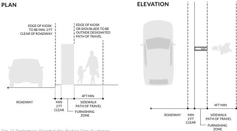
Fig. 11 Pedestrian-Oriented Wayfinding Sign Guidance
