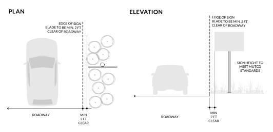
Fig. 8 Vehicular-Oriented Wayfınding Sign Guidance
