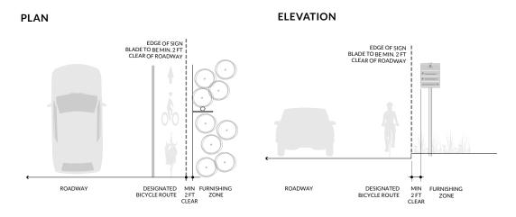
Fig. 10 Bicycle-Oriented Wayfınding Sign Guidance
