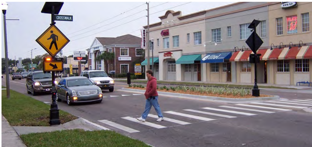
Figure 29. Rapid Flash Beacons - Photo courtesy www.pedbikeimages.org / Michael Frederick
