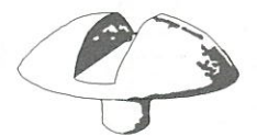
CONCRETE MUSHROOM GATE STOP INSTALLED ABOVE THE FINAL GRAVELED GRADE (INSTALL PER MANUFACTURER'S INSTRUCTIONS)
