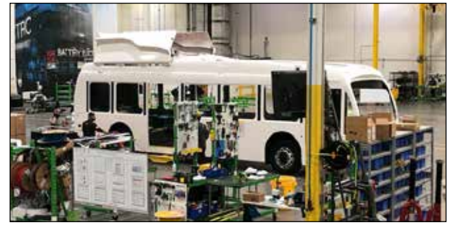
Bus manufacturer Proterra assembles a battery-electric bus for delivery to Wilsonville's SMART Transit.
