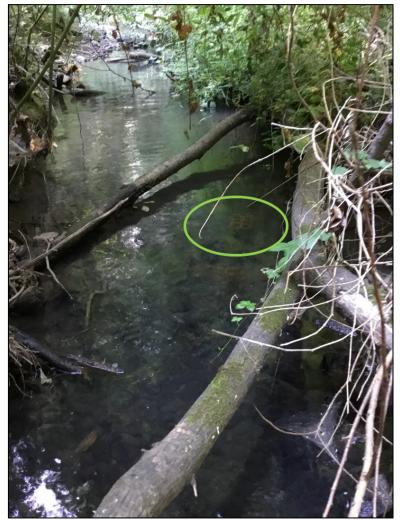
The green circle on the photo above shows the brick that the temperature loggers are strapped to and placed in Boeckman Creek.
