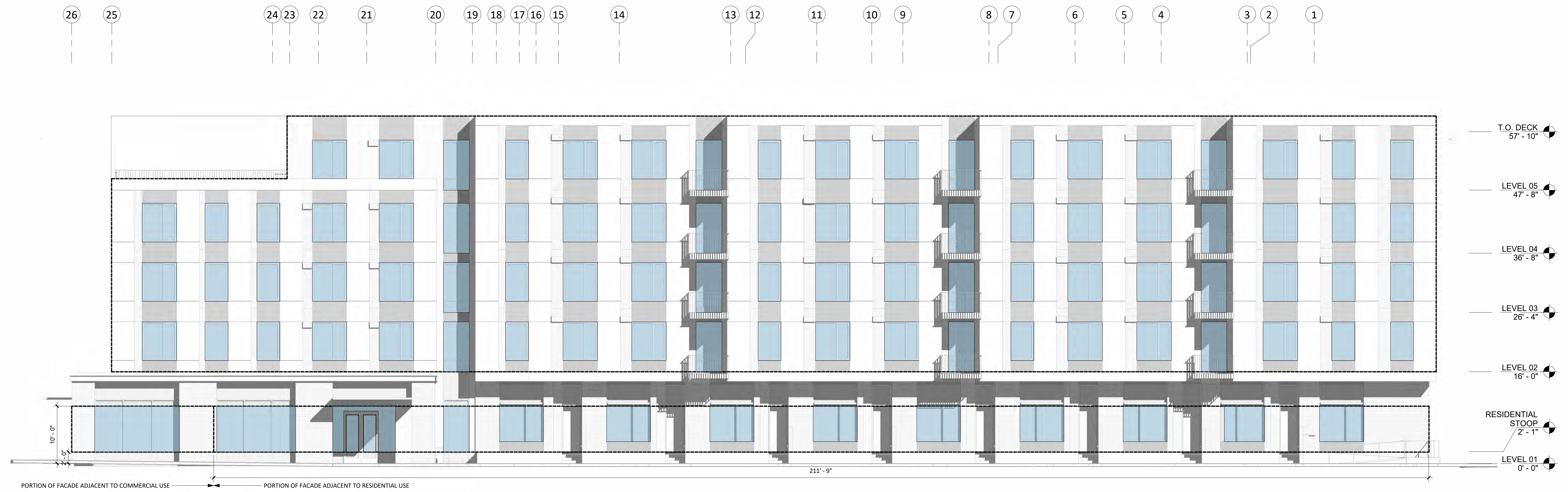
3 NORTHEAST ELEVATION - WINDOW AREA
