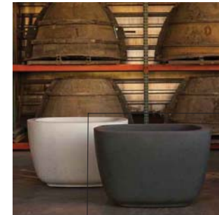
PRECAST CONCRETE PLANTER MANUFACTURER: LANDSCAPE FORMS MODEL: LARKSPUR - 30" STYLE: 30" IS 48" SQ. HOLDS APPROX. 17 CUBIC FEET OF PLANTING MATERIAL COLOR: GRAPHITE SIZE: 48"Dx48"Wx30"H SEE DETAIL 2 SHEET DLT3 FOR IRRIGATION CONNECTION
