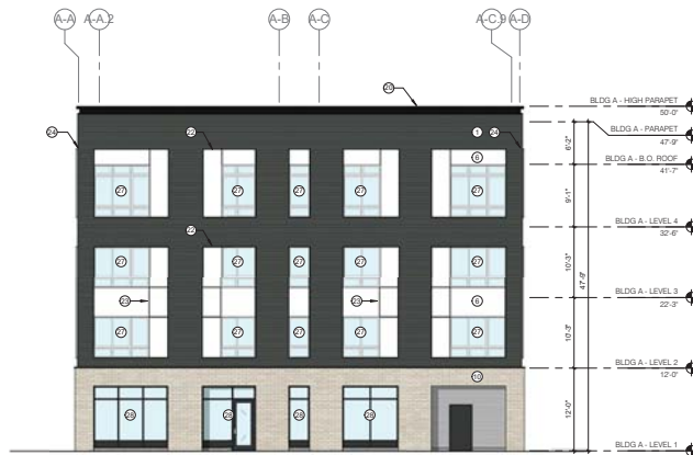
2 BLDG A - ELEVATION - SOUTH 1/8" = 1'-0"
